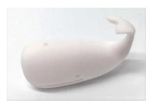
carbonating coating develops on the surface of the part, isolating the plastic below. In addition, the material has a higher stiffness compared to regular PA12. Typical applications are where flame retardant behaviour is required, i.e. in the aviation and electronics industry.
