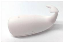
Oceanz PAFR is a polyamide material with a halogen free, chemical flame retardant. In case of a fire, a carbonating coating develops on the surface of the part, isolating the plastic below. In addition, the material has a higher stiffness compared to regular PA12.
