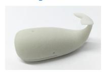
Oceanz PAGF is a glass-filled whitish polyamide 12 powder, which is characterized by an excellent stiffness in combination with good elongation at break. Laser sintered parts made from Oceanz PAGF possess excellent material properties:
