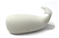
PA11 is a bio-based whitish polyamide material. Compared to PA12 it offers a higher elongation at break, elasticity and impact resistance. Typical applications are therefore environments where high deformations occur. In addition, the material does not splinter when
