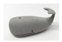
Oceanz Alumide is a metallic grey, aluminium filled polyamide 12 powder, which is characterised by its high stiffness, metallic appearance and good postprocessing abilities. Laser sintered alumide parts are characterised by:
